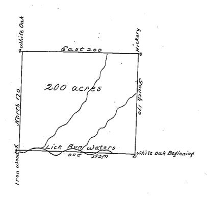
The above is a Draught of a Survey made in the month of July 1785 In Priserance of Instruct ions from the Surveyor Genl Dated the 22d Day of Jan 4 1785 Situate on the North Side of the Ohis sin the waters of the Dick Pun in Destrict No. 2. Containing two hundred Acres with allowance of 6 plaint.
